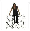
Step 1 Remove frames (A) from cases. Standing in front or behind expand the frames (A) by pulling up from the middle of the frame.
